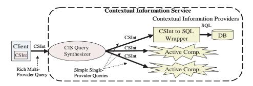
Figure 1. The CIS architecture
